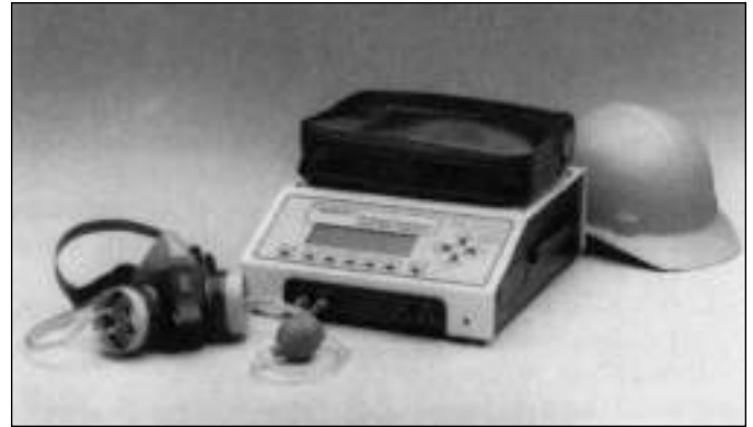
Figure 22-39. This quantitative fit-test equipment determines leakage by creating a negative pressure inside the facepiece similar to normal inspiratory pressures and measuring the leakage rate of air. (Courtesy Occupational Health Dynamics.)
