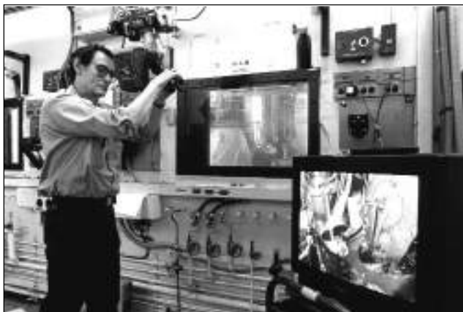
Figure 10–19. Use of a remote camera and external video screen for viewing areas in a hot cell.
