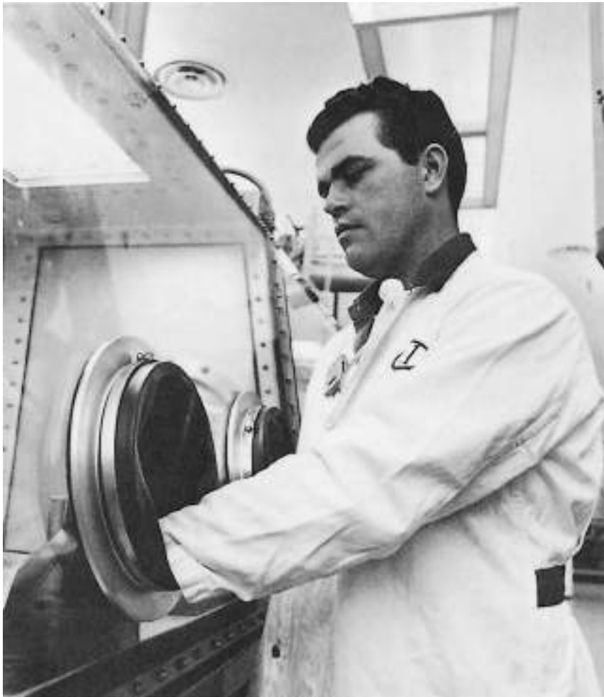
Figure 18-7. Some operations require complete enclosure. Here, a technician works with aluminum powder, used in atomic reactor fuel elements, at a glove box. He is wearing a film badge and air sampler on his lapel.
