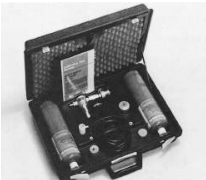
Figure 17-29. A calibration test kit for calibrating combustible gas and toxic gas sensors or instruments. (Courtesy MSA.)
