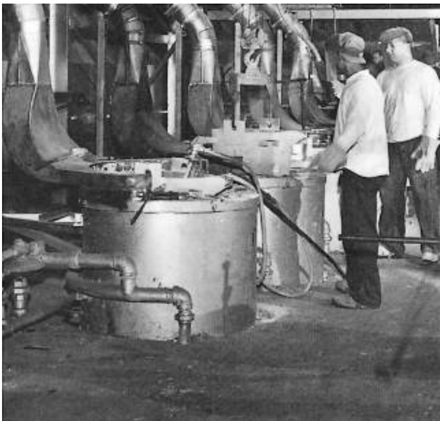
Figure 18-9. The fumes arising from lead-melting operations are controlled by local lateral-slot exhaust ventilation. (Courtesy Ford Motor Co.)
