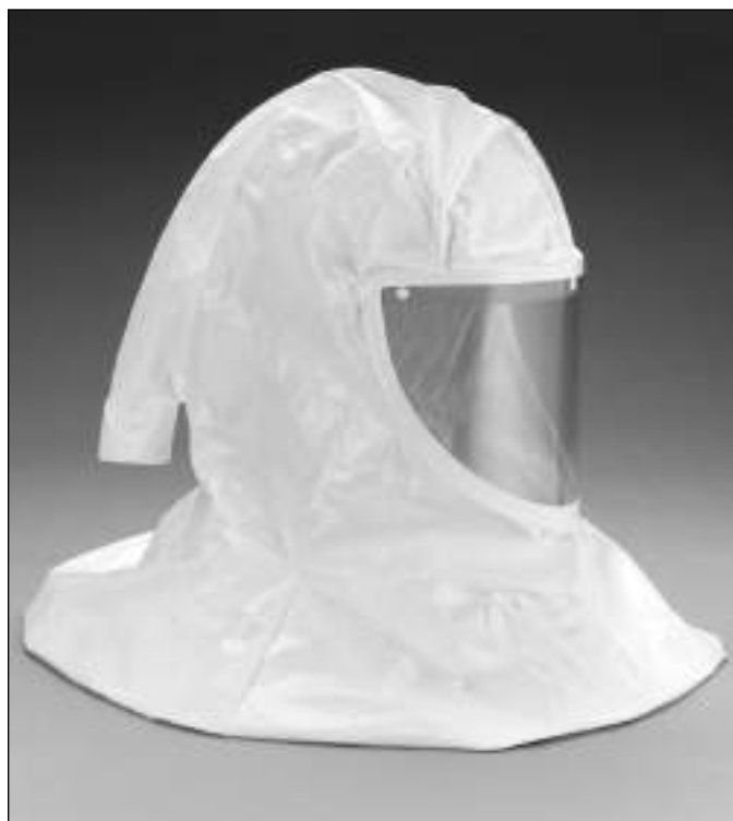
Figure 22-2c. The three types of loose-fitting respiratory inlet coverings: a. Loose-fitting facepiece. b. Helmet. c. Hood. Respirators with loose-fitting respiratory inlet coverings do not need to be fit tested. The loose-fitting facepiece is not suitable for workers with beards because it forms a partial seal with the face. The loose-fitting helmet (b) and hood (c) are acceptable for workers with beards. (Courtesy 3M.)
