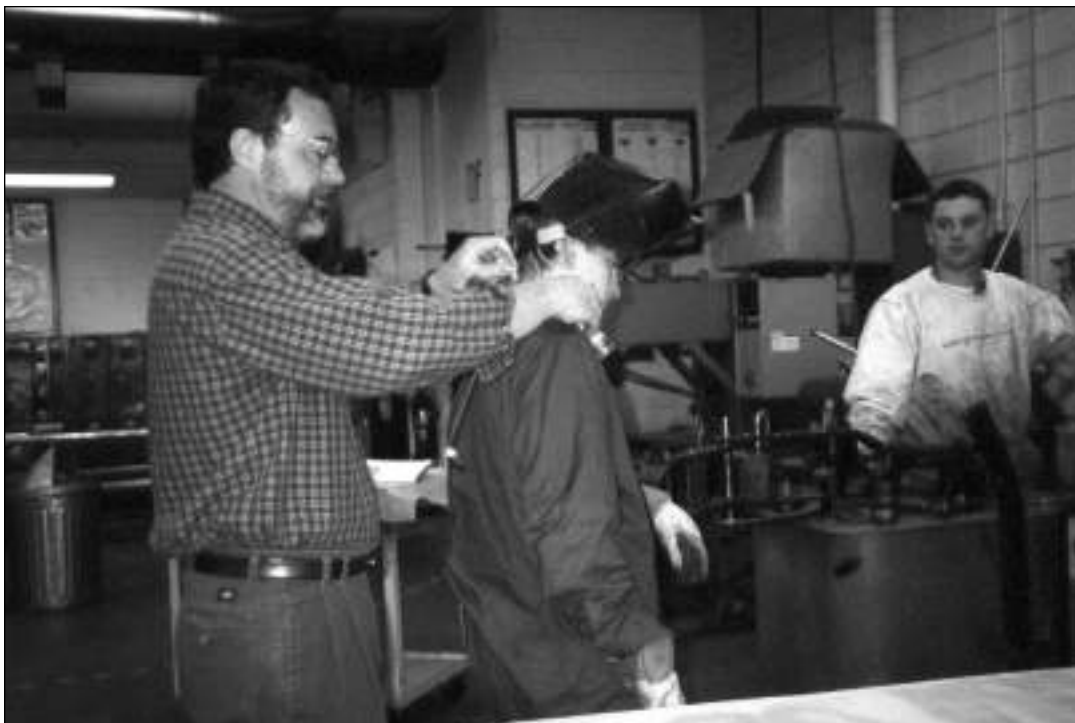
Figure 15–3. In personal monitoring, the measurement device, or dosimeter, is placed as close as possible to the contaminant's route of entry into the body. For example, when monitoring an air contaminant that is toxic if inhaled, the measurement device, or dosimeter, is placed on the employee's lapel or as close to the breathing zone as possible. When monitoring noise, the dosimeter should be placed close to the ear. (Photo by Elise Pechter)
