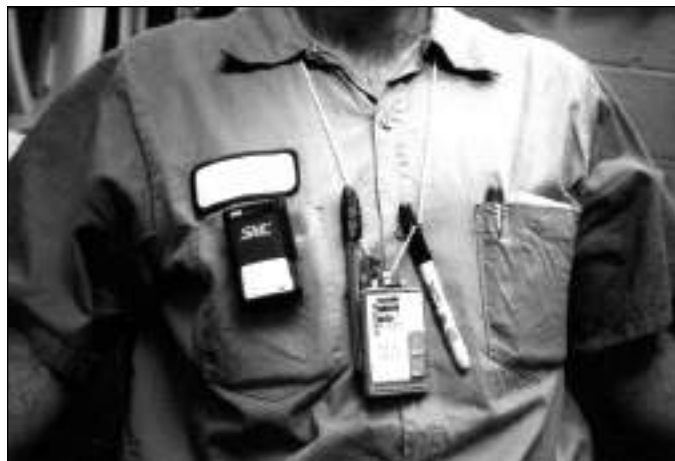
Figure 10-8. A health physics technician wearing a thermoluminescence detector attached to a neck strap and an electronic alarming dosimeter on his right shirt pocket.
