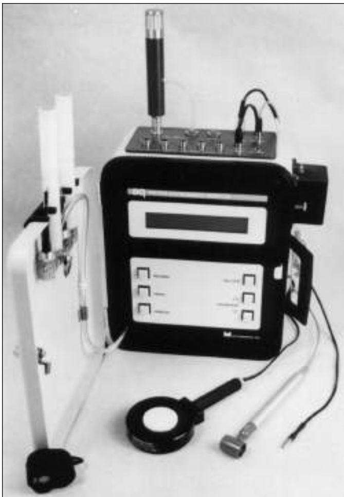
Figure 17–11. An indoor environmental monitor for measuring temperature, relative humidity, carbon dioxide, and one other parameter. (Courtesy Metrosonics, Inc.)
