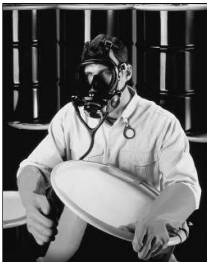
Figure 22–21. A continuous flow air-line respirator with a tight-fitting facepiece. (Courtesy 3M.)
