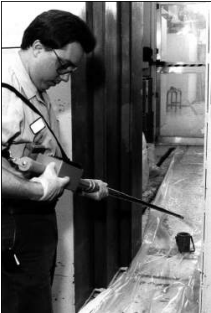
Figure 10-10. Health physics technician using telescopic high-range ion chamber survey instrument. (Note the thermoluminescent dosimetry badge on shirt pocket and electronic alarm dosimeter on trouser pocket.)
