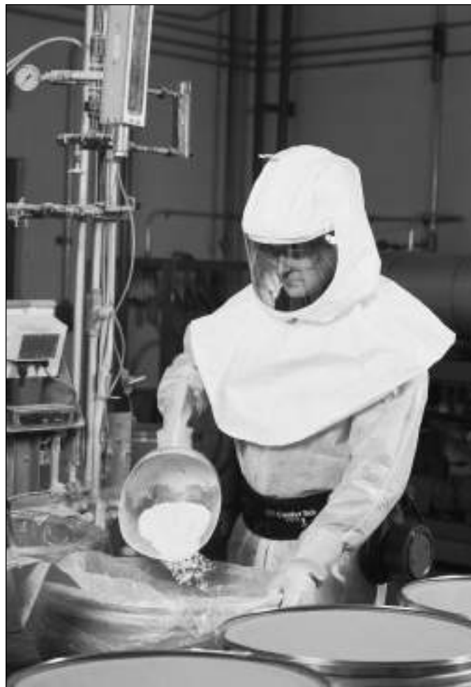
Figure 22-18. Powered air-purifying respirators with hoods or helmets can be worn by workers with beards and/or eyeglasses. (Courtesy 3M.)
