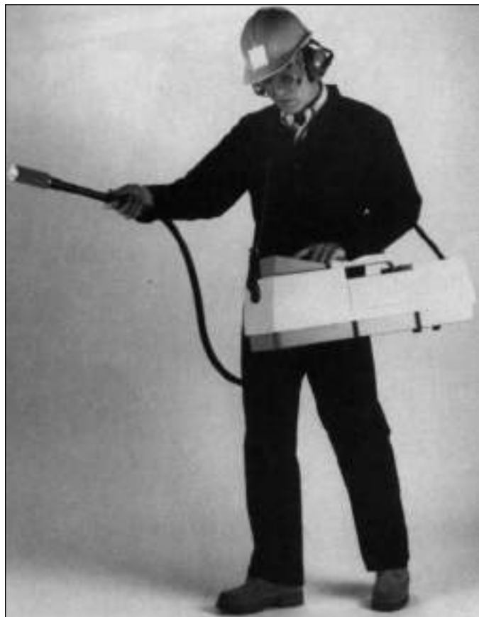
Figure 15–8. This portable ambient air analyzer can be used to measure concentrations at the operator's workstation. (Courtesy Foxboro Co.).
