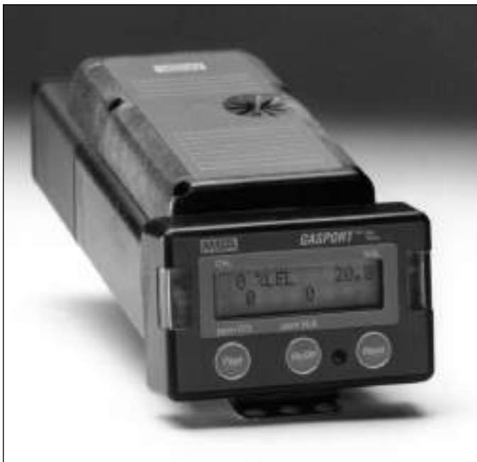
Figure 17-5a. A Gasport® combustible gas monitor. (Courtesy MSA.)
