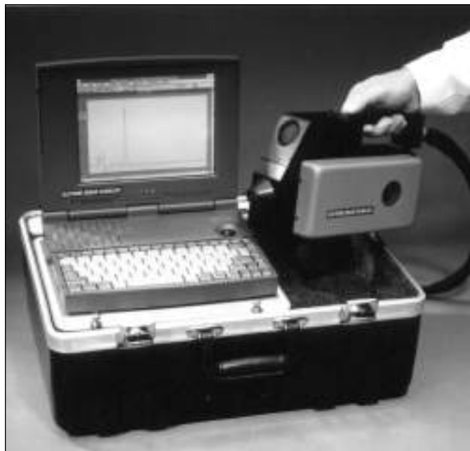
Figure 17–24. A hand-held, preprogrammed gas chromatograph that uses a surface acoustic wave detector. (Courtesy Electronic Sensor Technology.)
