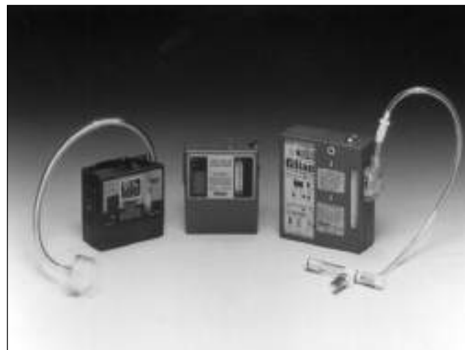
Figure 16–13. Personal sampling pumps must be lightweight and easy to use. (Courtesy Gillian Instrument Corp.)
