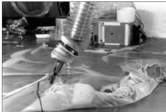
Figure 10–20. Remote removal of strippable decontamination paint in a hot cell.
