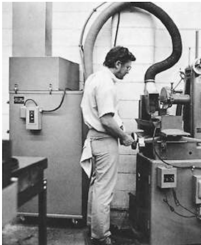
Figure 18–10. A typical local exhaust ventilation system—a dust collector—traps contaminants near their source, so the worker is not exposed to harmful concentrations.
