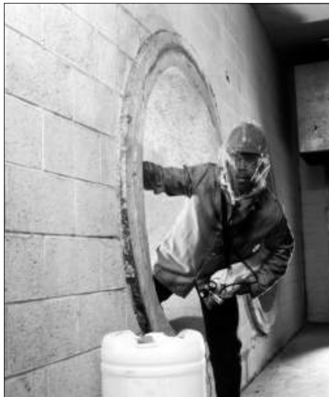
Figure 22-26. Some self-contained breathing apparatus are designed for escape-only from hazardous atmospheres. (Courtesy MSA.)
