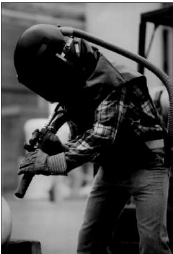
Figure 22-23. Abrasive blasting continuous flow air-line respirator. (Courtesy 3M.)
