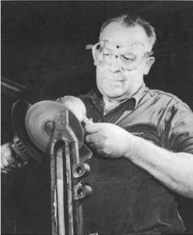
Figure 5-8. Flexible-fitting goggles should have a flexible frame forming the lens holder.
