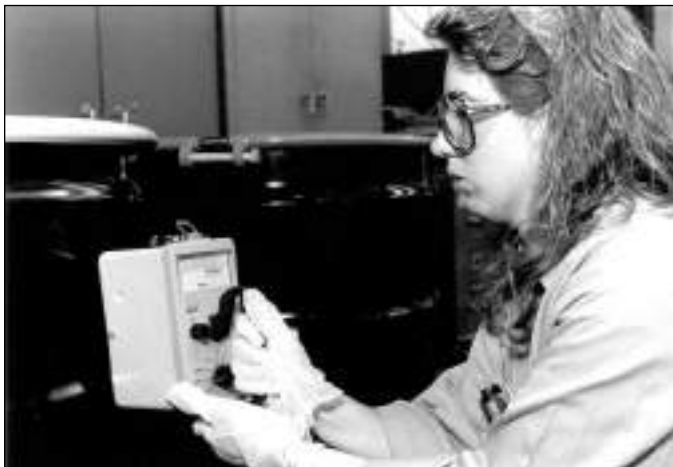
Figure 10-11. Health physics technician taking exposure rate readings with an ion chamber survey instrument.
