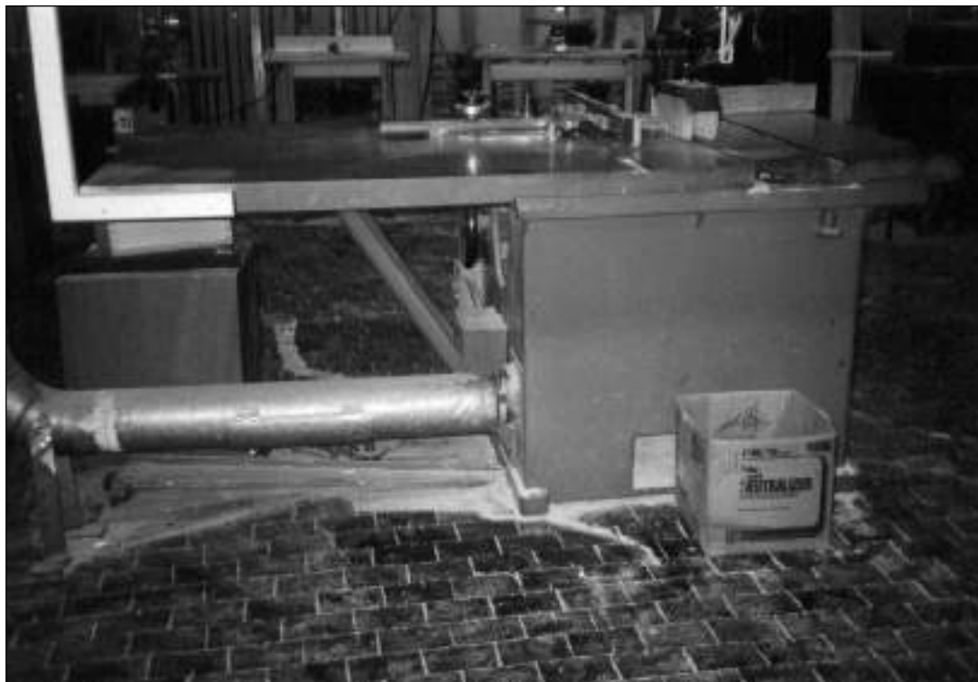
Figure 15-2. Observing dusty operations, patterns of shavings or powder on the floor, overspray on walls, puddles underneath valves, or wetness around an area not currently in use alerts the industrial hygienist to problems not considered before. The pattern of wood dust under this saw indicated that the local exhaust ventilation was disconnected. (Photo by Elise Pechter)
