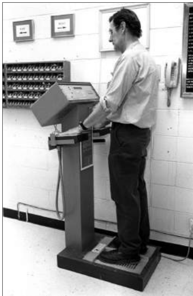
Figure 10–18. Use of a hand-and-shoe monitor for final radiological checkout.
