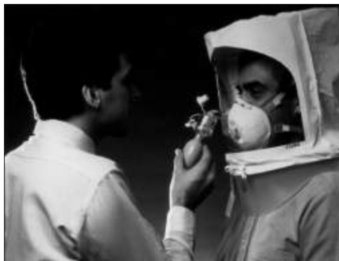
Figure 22-34. The saccharin qualitative fit test can be used with any particulate or gas/vapor respirator with any particulate filter to determine adequacy of fit. (Courtesy 3M.)
