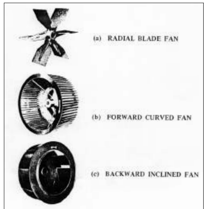
Figure 19-8. Common types of centrifugal fans. (Source: McDermott, 2000.)
