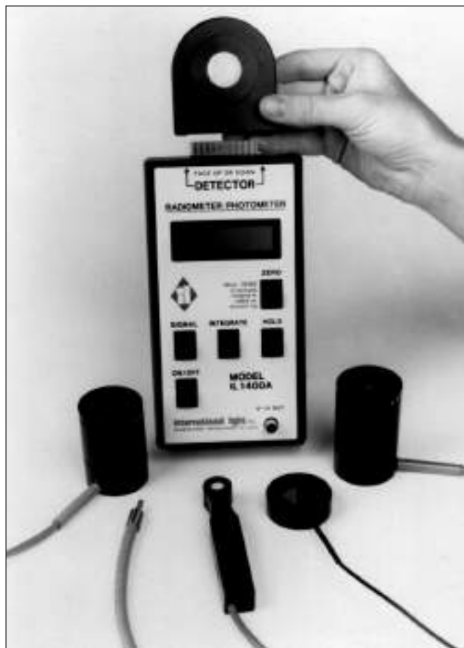
Figure 11–21. Instruments are now on the market that have wavelength response characteristics that approximate the spectral effectiveness curves of the TLVs. (Courtesy International Light, Inc.)
