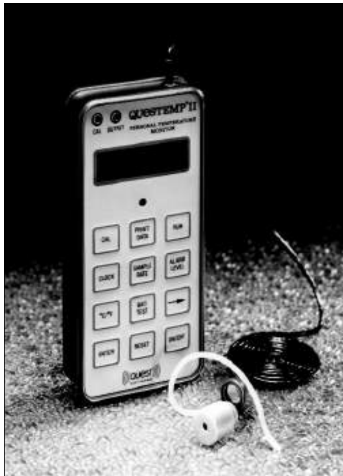
Figure 12–10. Photographs of two commercially available personal monitors developed for heat-stress exposures. (Courtesy of Metrosonics, Inc, and Quest Technologies.)
