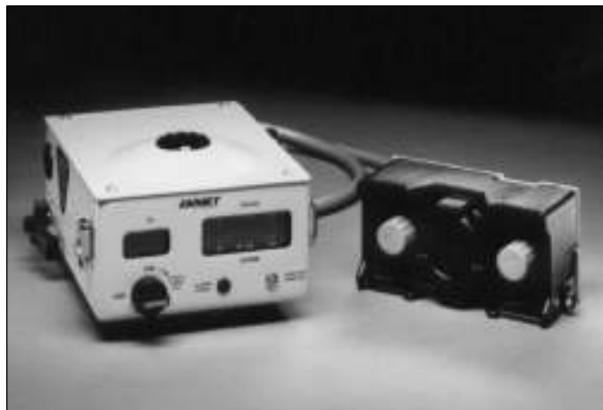
Figure 17-3. A multigas monitor that uses a metal oxide semiconductor detector to measure combustible gases. A detachable sensor head for remote sampling is one feature of this instrument. (Courtesy ENMET Corporation.)
