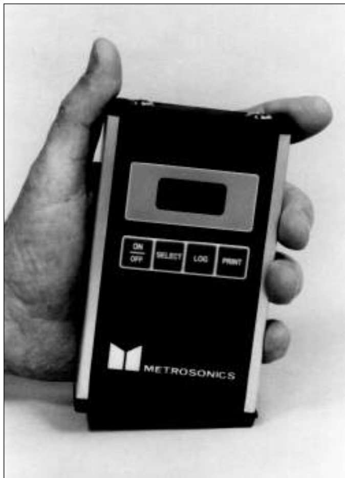
Figure 12–10. Photographs of two commercially available personal monitors developed for heat-stress exposures. (Courtesy of Metrosonics, Inc, and Quest Technologies.)
